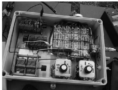
Figure 8 — G3RCQ's phasing box. C1 is at the lower left, with redundant X_p components above
